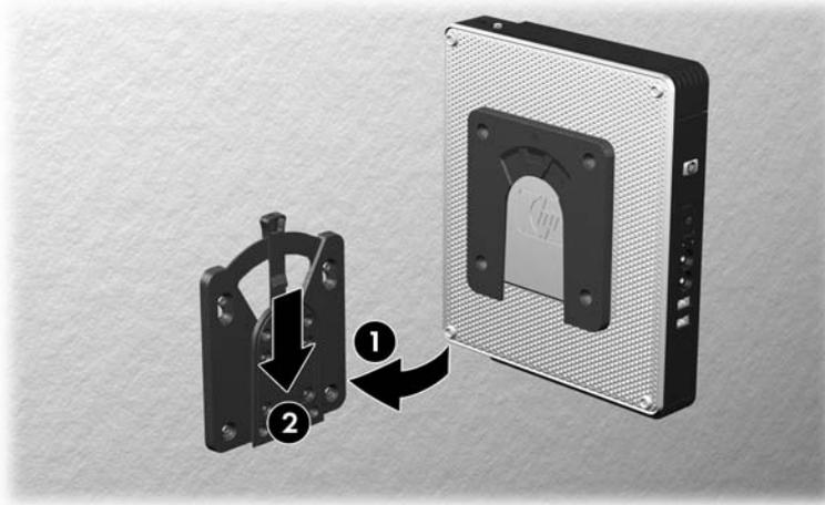
**NOTE:** When attached, the HP Quick Release automatically locks in position. You only need to slide the lever to one side to remove the thin client.
