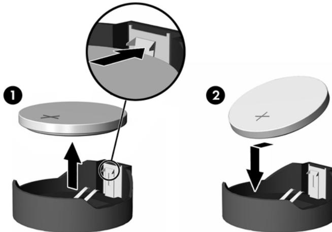
3. To insert the new battery, slide one edge of the replacement battery under the holder's lip with the positive side up. Push the other edge down until the clamp snaps over the other edge of the battery (2).
