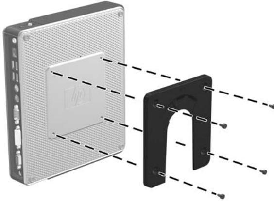
2. Using four screws included in the mounting device kit, attach the other side of the HP Quick Release to the device to which you will mount the thin client. Make sure the release lever points upward.
