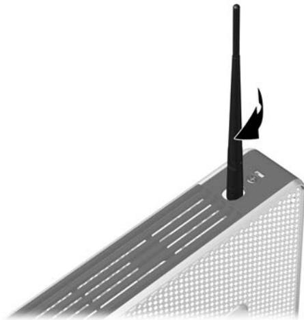
△ **CAUTION:** To prevent damage to the antenna mounting, do not overtighten the antenna.
